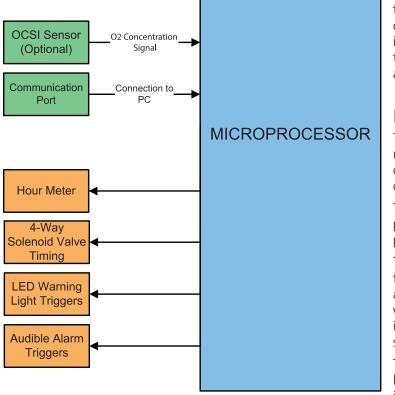
Figure 5: Microprocessor Operation Block Diagram
