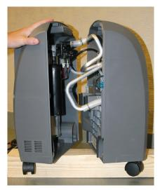
3. Using pliers to remove the spring clamps holding the braided tubing to the 4-way solenoid.
