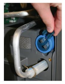
4. Pull upward to remove capacitor.
