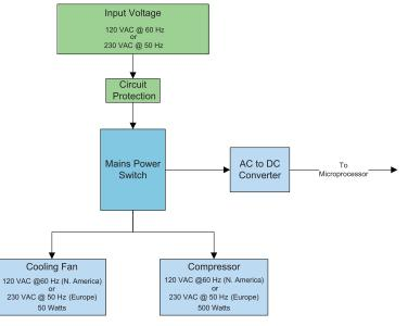
Figure 4: Diagram of Mains Electrical Distribution
