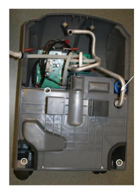
6. Disconnect the black hose from the intake on the compressor.
