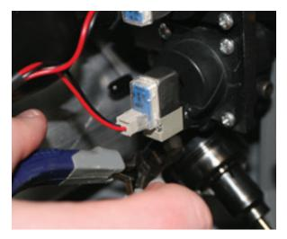
6. Disconnect both the 4-way solenoid and power cord electrical wires from the main circuit board
