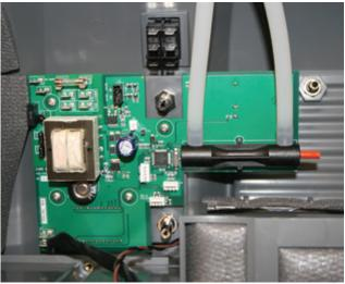
PCB connections & Mounting Screws
