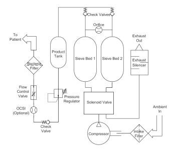
Figure 3: Schematic Diagram of Pneumatic Operation
